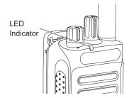
NOTE: The LED lights up solid green while the radio is transmitting and double blinks green when the radio is receiving a privacy-enabled call.
