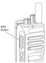
While a call is in progress, the **PTT** button allows the radio to transmit to other radios in the call.
