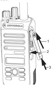
Insert the slanted end of the cover into the slots above the universal connector. Press downward on the cover to seat the dust cover properly on the Universal Connector.
