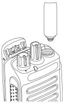
To remove the antenna, turn the antenna counterclockwise.
