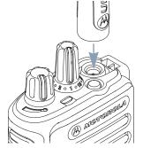
To remove the antenna, turn the antenna counterclockwise.
