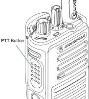
While a call is not in progress, the PTT button is used to make a new call (see *Making a Radio Call* on page 18).
