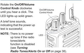
If your radio does not power up, check your battery. Make sure that it is charged and properly attached. If your radio still does not power up, contact your dealer.
