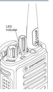
**Blinking green** – Radio is receiving a non-privacy-enabled call or data, or detecting activity or retrieving Over-the-Air Programming transmissions over the air.
